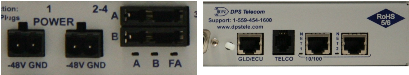
Back panel LEDs for Power (left) and Ethernet connections
