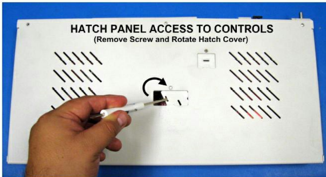
Hatch Panel Access on Top of the NetMediator RTD G5 Chassis
