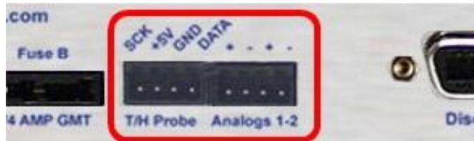
*Fig. 6.5.4.1. Temperature Sensor and Analog Connectors*
