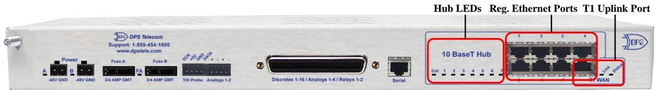
Fig. 6.8.1. NetGuardian integrated Ethernet Hub
