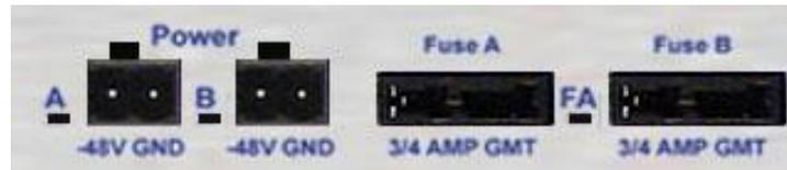
*Fig. 6.3.1. Power connectors and fuses*
