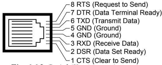
**Fig. 6.6.2.** Serial (Yost) port pinout
