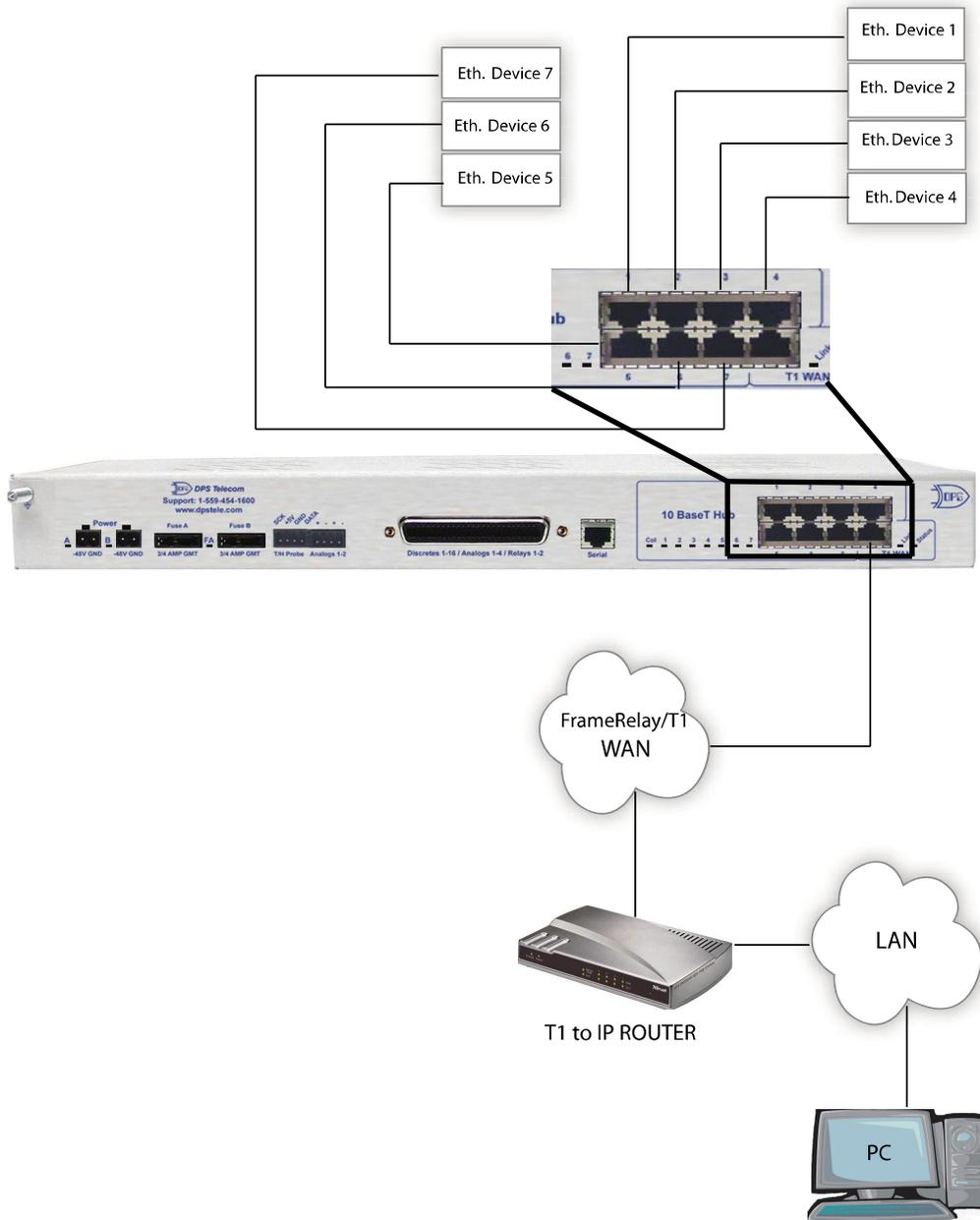
*Fig. 6.4.1. Chart of Ethernet and T1 WAN Connections*
