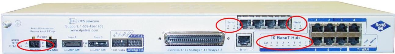
*Fig. 8.1. Back panel LEDs for Power and Ethernet connections*
