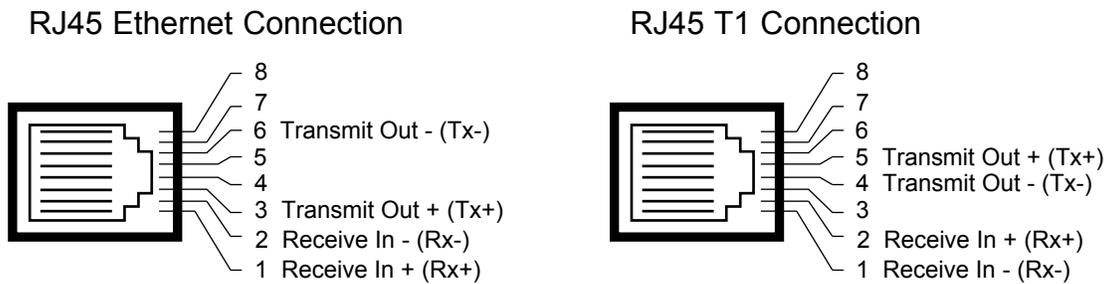
**Fig. 6.4.2** Ethernet ports and T1 WAN port pinouts
