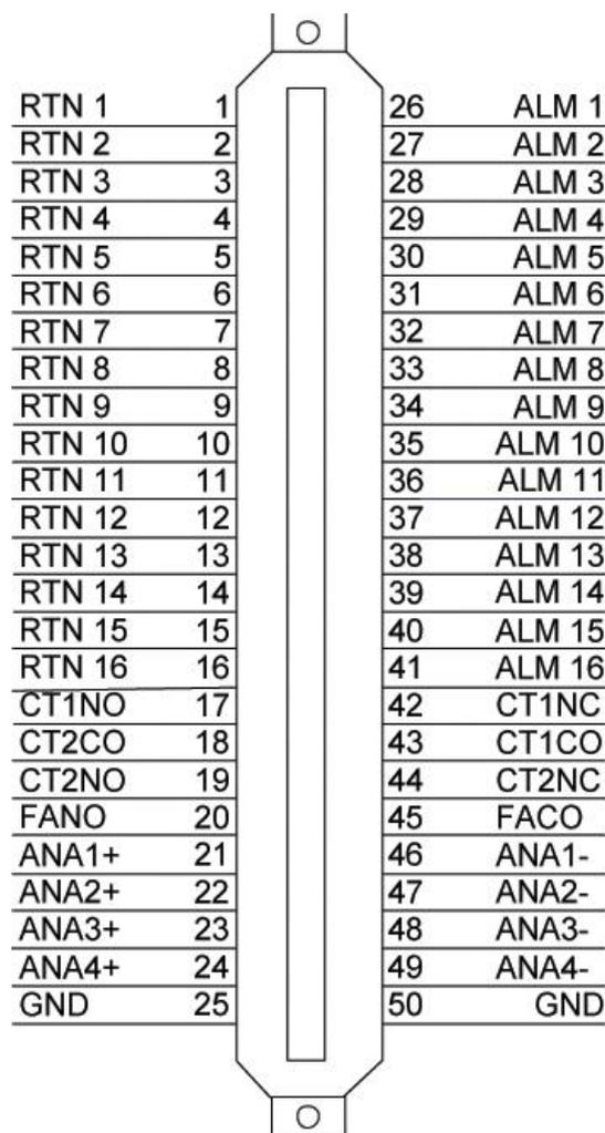
*Fig. 6.5.2.. Pinout Diagram for Discretes 1-16 connector*
