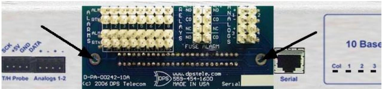
**Fig. 6.7.1.** The wire-wrap back panel (arrows indicate screw locations for mounting)
