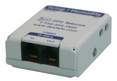
Daisy-chain up to 15 of these rugged sensors from your NetGuardian. Both power and communication are handled by a simple RJ-12 cable. A variety of sensors are available, including temperature, humidity, and battery voltage.
