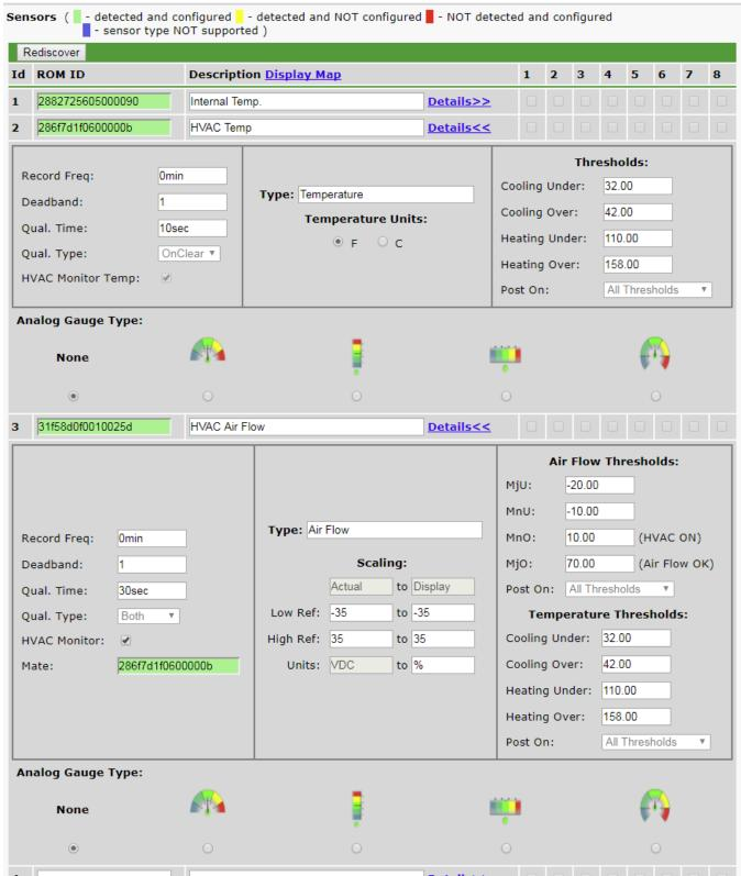
Sensor with HVAC Monitoring enabled.
