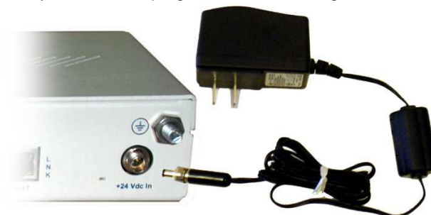
Fig. 5.3 Close-up view of NetGuardian's screw-on power connector.
