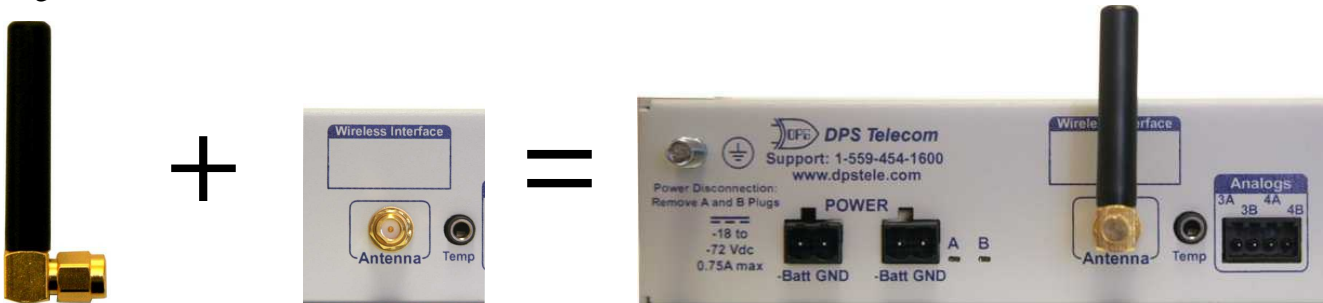
The Antenna attaches to the NetGuardian's back panel to facilitate cellular signal reception
