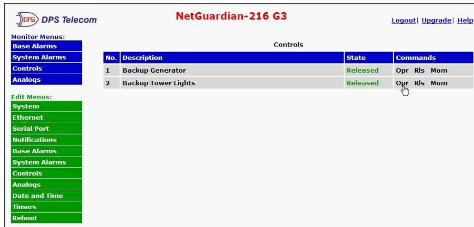
Fig. 11.23 Operate the control relay by clicking on one of the actions in the Commands field.
