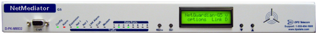
Fig. 1.1. NetMediator TNT G5 monitors alarms, pings network elements, and reports via SNMP, pager, or email
