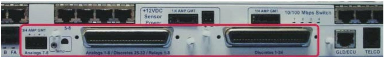
*Fig. 6.6.1. Alarm and control relay connectors*
