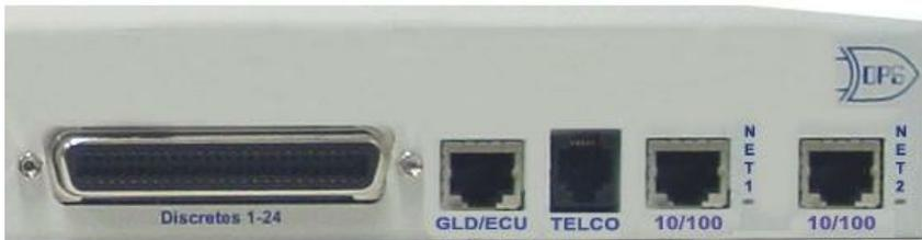
*Fig. 6.4.2. Two 10/100 Ethernet ports (Without Switch)*
