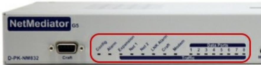
*Fig. 9.1. Front panel LEDs*
