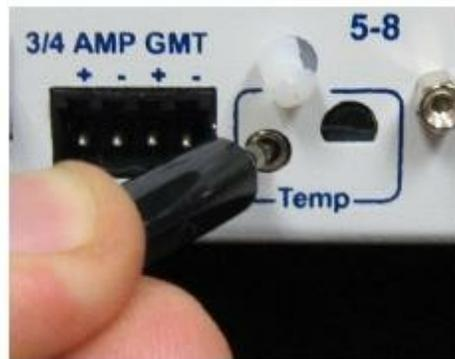
*Fig. 6.6.6.1. The external temperature sensor*
