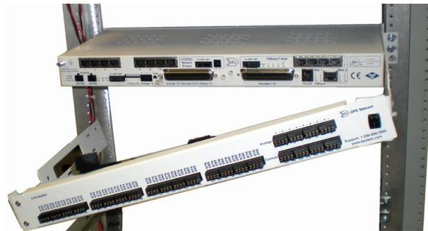
4. Close the back panel gate and lock it in place by turning the black swivel to the vertical, locked position as indicated on the silk screen (See Figure 6.14.1).
