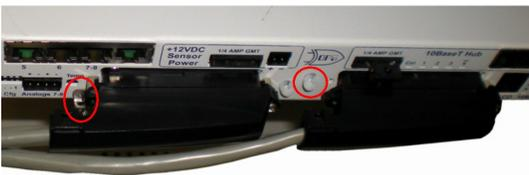
7. Tighten the 2 screws located to the right of the amphenol cables. Use the plastic zip ties provided to secure both cables to the NetMediator where shown (bottom image). **Note:** A zip tie will be used on the NetMediator's small metal tab to secure the left amphenol cable. If your remote is equipped with the 4-pin analog connector, connect it to the NetMediator **and** to the DB9 on the hinged panel.
