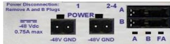
*Fig. 6.3.1. Power connectors and fuse.*
