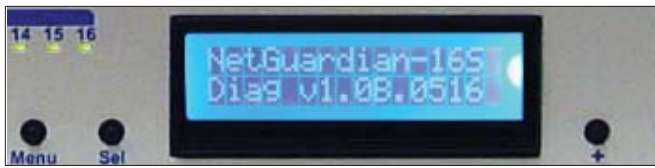
Integrated Building Status Unit provides local audiovisual notification
