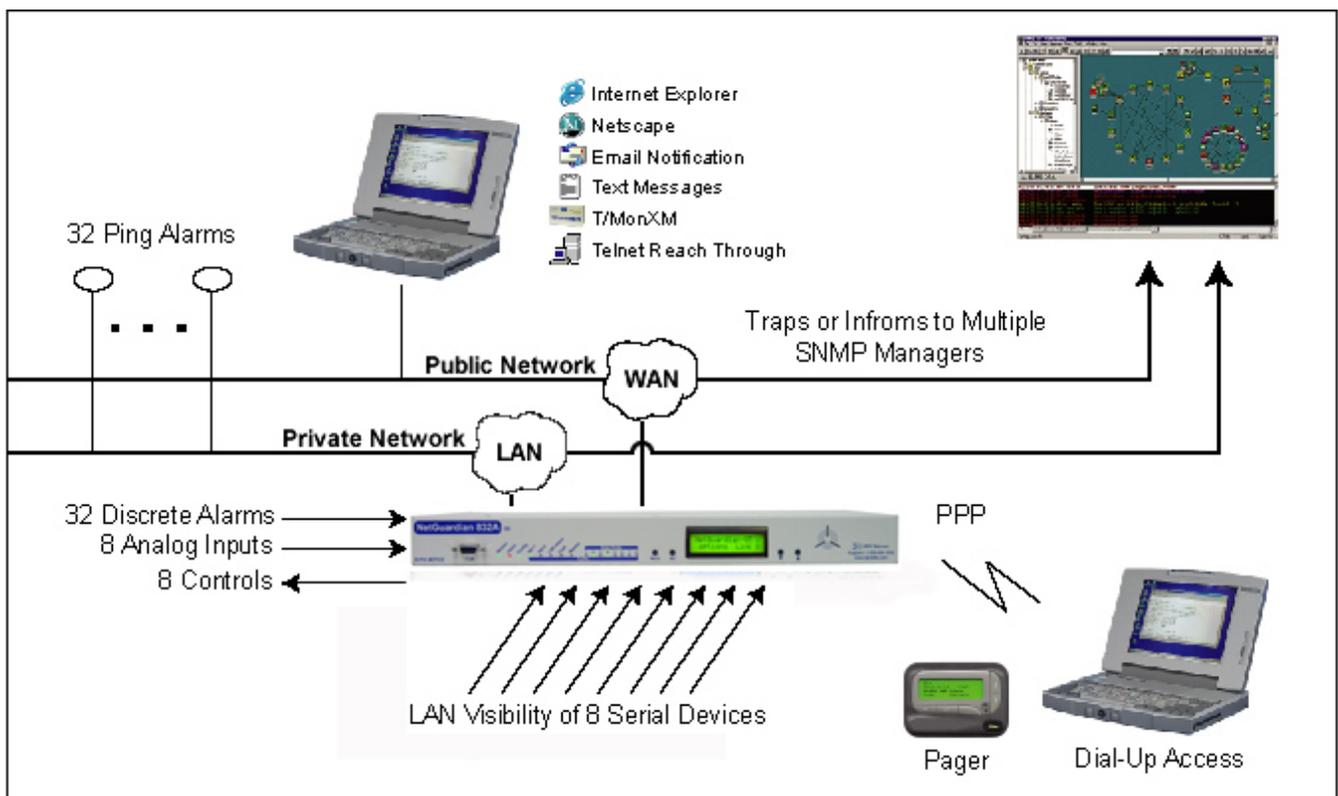
**Fig. 1.2.** NetGuardian 832A G5 has the capacity to monitor IP aware devices' network presence and also interfaces discrete alarm points and controls at your network sites
