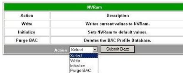
*Fig. 2.42. NVRAM enables the NetGuardian to retain data even through a power loss*
