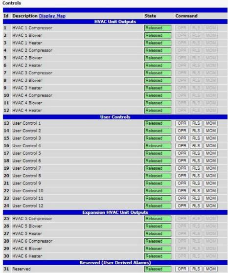
View and operate control relays from the Monitor > Exp. Controls menu
