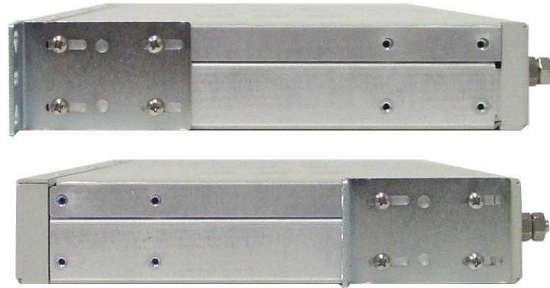
Cell16 can be flush or rear-mounted
