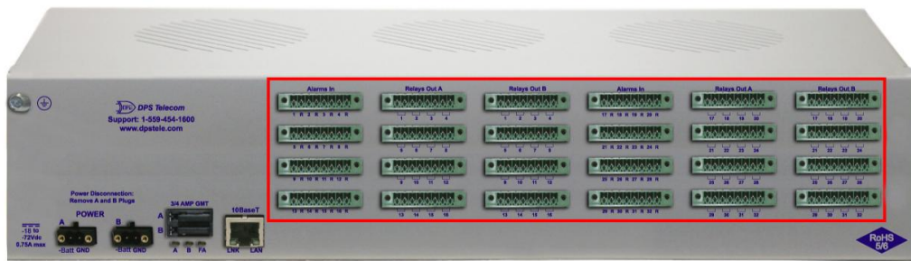
Fig 5.4 Alarm and Relay ScrewLug Connectors
