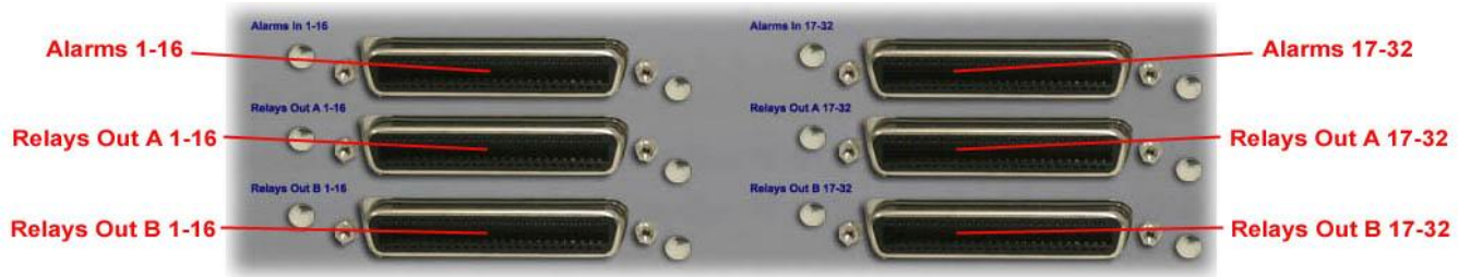
Fig 5.7a Alarm and Relay Amphenol Connectors
