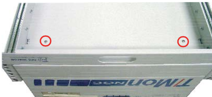
Fig. 1.1 - These screws secure the T/Mon to the Slide Rack
