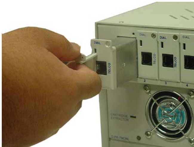
Fig. 1.15 - Use the Cartridge Extractor to remove the old Port Interface Cartridge
