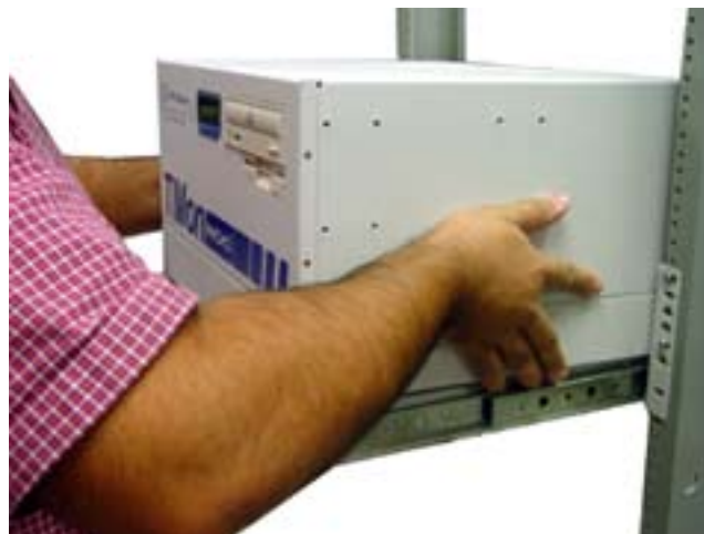
Fig. 1.3 - Place the T/Mon on the extended Slide Rack
