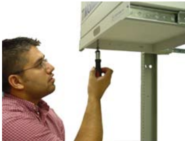
Fig. 1.5 - Secure the T/Mon by inserting the two mounting screws from below
