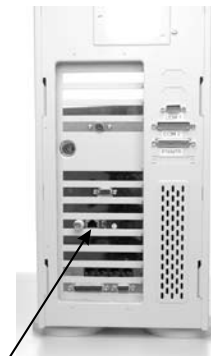
Fig. D.4 - Follow these steps to install an Ethernet card in a T/MonXM tall tower case
