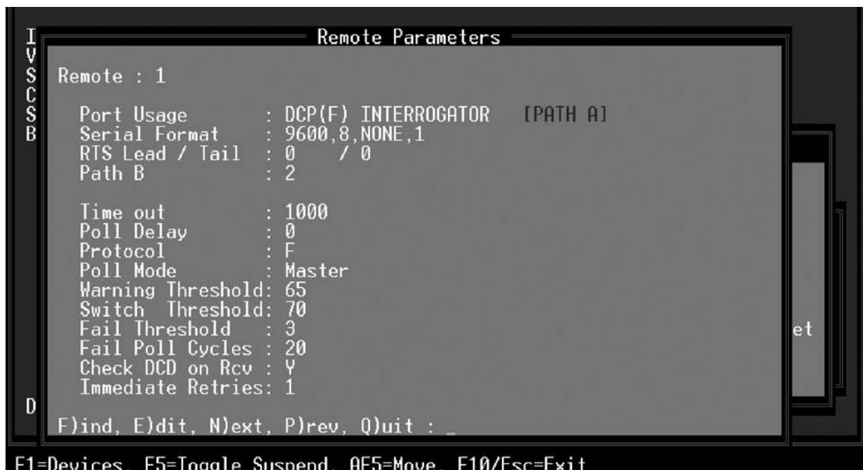
Fig. M1.34 - Enter a remote port number for Path B in the DCP(F) Interrogator Definition Screen
