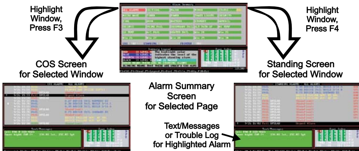
Fig. 17.2 - Monitor mode shows alarm details in COS and standing alarm screens.
