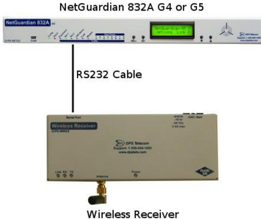
1. Insert one end of the RS232 serial cable into the Serial Port input on the wireless receiver.
