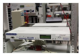
1. To begin installing the hinged pluggable back panel, the NetGuardian 864A should be removed from rack if already mounted in rack. Remove rack ears as well.
