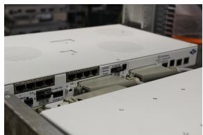
3. Attach Hinged Surge Panel onto rear of 864A, the side with 2-50 pin connectors will face the 864A, the 4-50 pin connectors will face outward to connect to external equipment.
