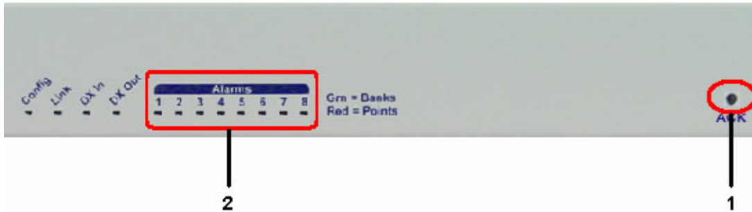
Fig. 3.1. The front panel displays alarm and communication status.
