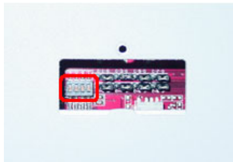
Fig. 2.4.5.1. Shelf addressing DIP switch close-up.
