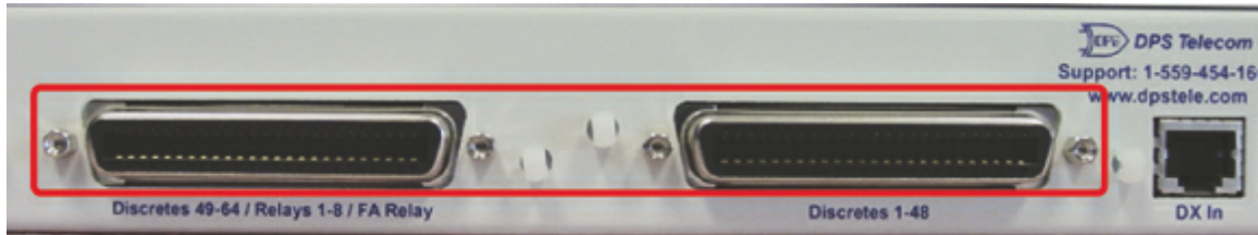
Fig. 2.4.6 Alarm and control relay connectors
