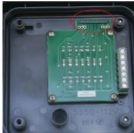
Put the two pieces back together. First, on the inside cover, locate the 10-pin male connector. This connector will need to correspond to the 10-pin female connector on the board on the base unit (image below).
