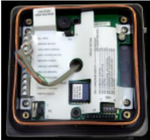
From the inside of the unit, locate the screw connectors. This is where you'll attach the wires to the RJ45 connector.
