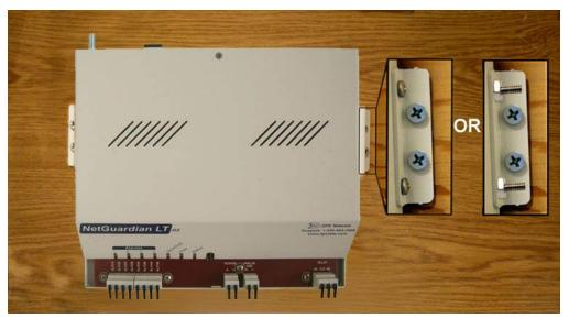
*Fig 5.2* Use the included wall mount bracket to mount the NetGuardian LT vertically on the wall. Wall-Mounting Instructions
