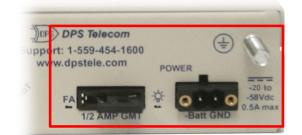
The NetGuardian LT G2 is typically powered by a screw terminal barrier plug connector, but other options exist.
