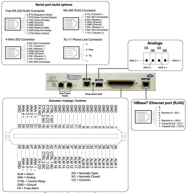
Fig. 5.1 NetGuardian 216 G3 back panel connections
