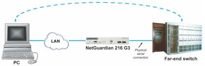
Fig. 11.4 - Topology of using the serial port for reach-through
