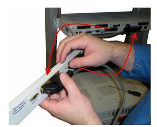
6. Unlock the back panel by turning the black swivel to the horizontal position. (See Figure 6.12.1) Plug the amphenol cables in to the hinged back panel and secure them with the Velcro straps. Make sure the NetGuardian's silk screen matches the hinged panel where the amphenols are connected.
