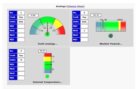
Fig. 11.25 - Monitoring analogs in Gauge View offers you a visual representation of where all your analogs stand.
