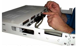
8. Use the remaining zip ties to keep the amphenol cords tied together. Trim the excess plastic off the zip ties with scissors.
