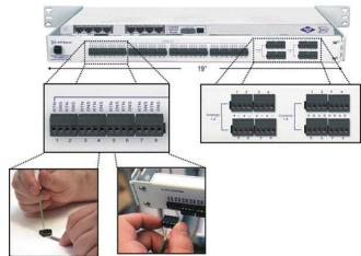
9. Close the back panel and lock it by turning the black swivel to the vertical position. **NOTE: The connectors on the Hinged Pluggable Back Panel support 18 - 26 AWG wire (stranded or solid). DPS recommends using 24 AWG wire (stranded).**
