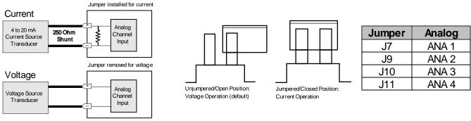
Fig. 5.7. Jumper settings for analog alarms inputs.
