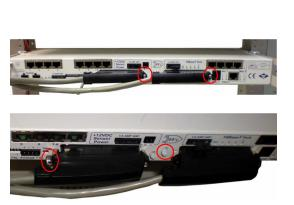
7. Tighten the 2 screws located to the right of the amphenol cables. Use the plastic zip ties provided to secure both cables to the NetGuardian where shown (bottom image). **Note:** A zip tie will be used on the NetGuardian's small metal tab to secure the left amphenol cable. If your remote is equipped with the 4-pin analog connector, connect it to the NetGuardian **and** to the DB9 on the hinged panel.
