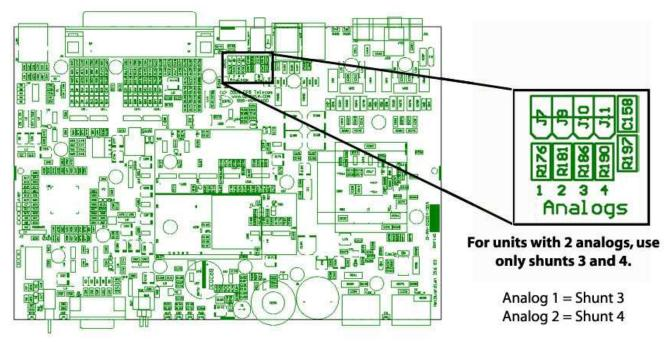
Fig. 5.6. Adjustable jumpers on the NetGuardian 216 circuit board
