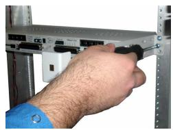
2. Facing the back of the NetGuardian, install the right side of the hinged pluggable back panel. Used the screws provided to secure the right mounting arm to the rack.
