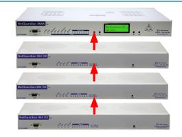
Hub: Alarm Point Inputs: Analogs: Control Outputs: Max. Voltage: Max. Current: Fuse: Operating Temp.: Operating Humidity: MTBF: 8 - 10BaseT ports with Uplink jack 32 (832 DX) or 64 (864 DX) 8 (max) Relay contacts, 8 each (max) Form A (N/O, N/C selectable) 60 VDC/120 VAC 1 Amp, AC/DC 1/4 Amp GMT 0° to 60°C (32° to 140°F) 0% to 95% non-condensing 60 years
