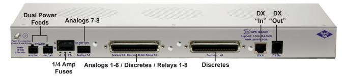
The back panel offers easy connectorization for power feeds, discrete alarms, relays, and 10BaseT hub.
