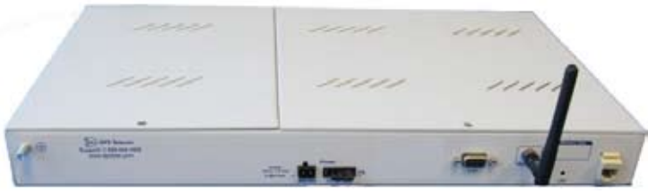
Back view of the NetDog 82 BW, featuring the wireless reporting option.
